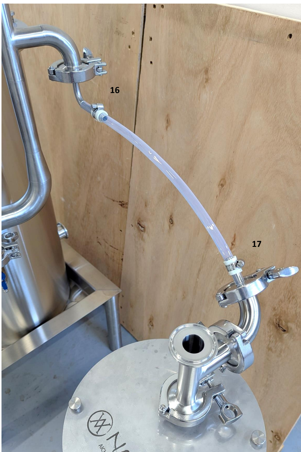
Picture 9: connecting the vacuum florentine flask to the Nano
