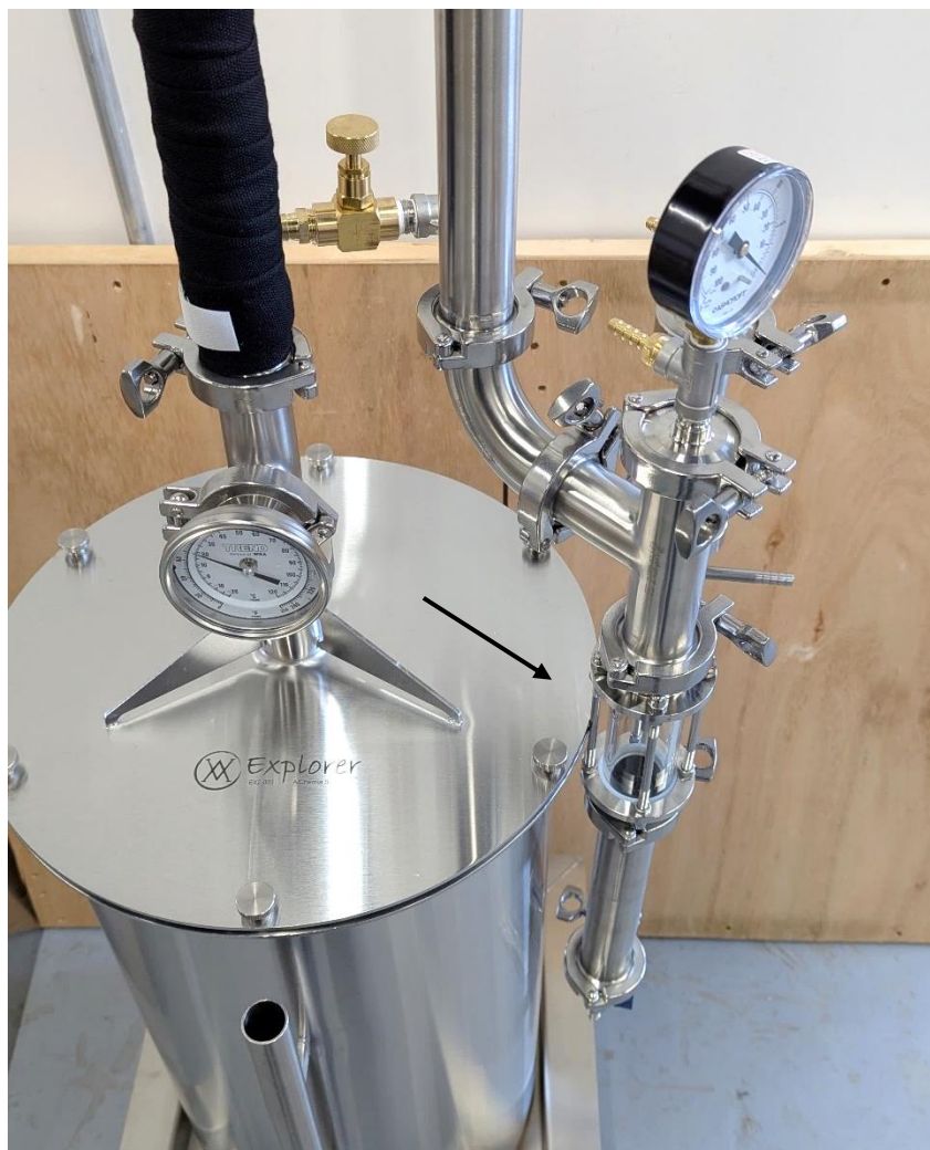
Picture 8: resting of the vacuum florentine flask against the Explorer flange and lid.
