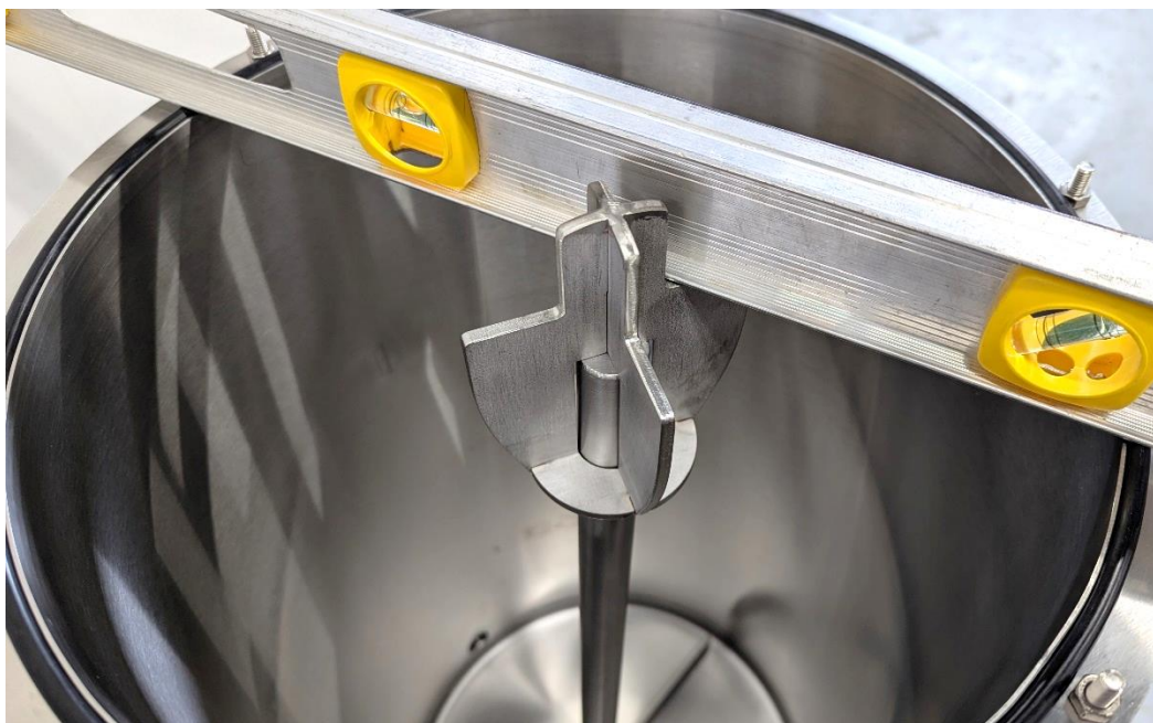
Picture 2: Pillar assembly in the tank. The pillar height must be adjusted so that anything flat rests on the pillar head AND on the O-ring on both sides of the tank.
